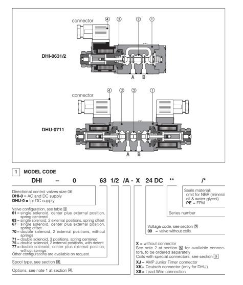
DHI and DHU are spool type, three or four way, two or three position direct operated solenoid valves designed to operate in oil hydraulic systems.
