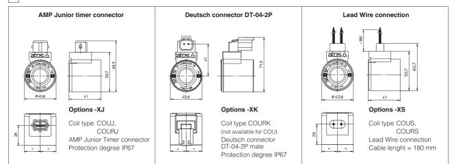
Note: The above coils are available only for voltage supply 12, 14, 24 and 28 VDC. For the characteristics refer to standard coils features - see sect.
