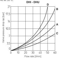
7 OPERATING LIMITS based on mineral oil ISO VG 46 at 50°C
