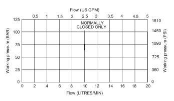
3-Way, 2-Position Spool 20 L/min (5 US GPM) Up to 100 bar (1500 PSI)
