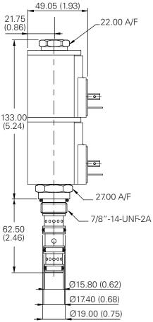
Ø15.80 (0.62) Ø17.40 (0.68) Ø19.00 (0.75) Installation drawing (Steel)
